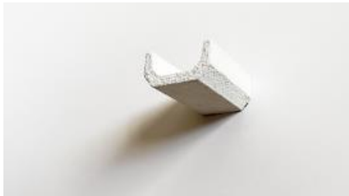
Figure 54 Elevation drawings of the rain-water draining system composed of water spout, water bowl and chain (above) and white exposed concrete water spout reproduction (below). (Produced by the author.)
