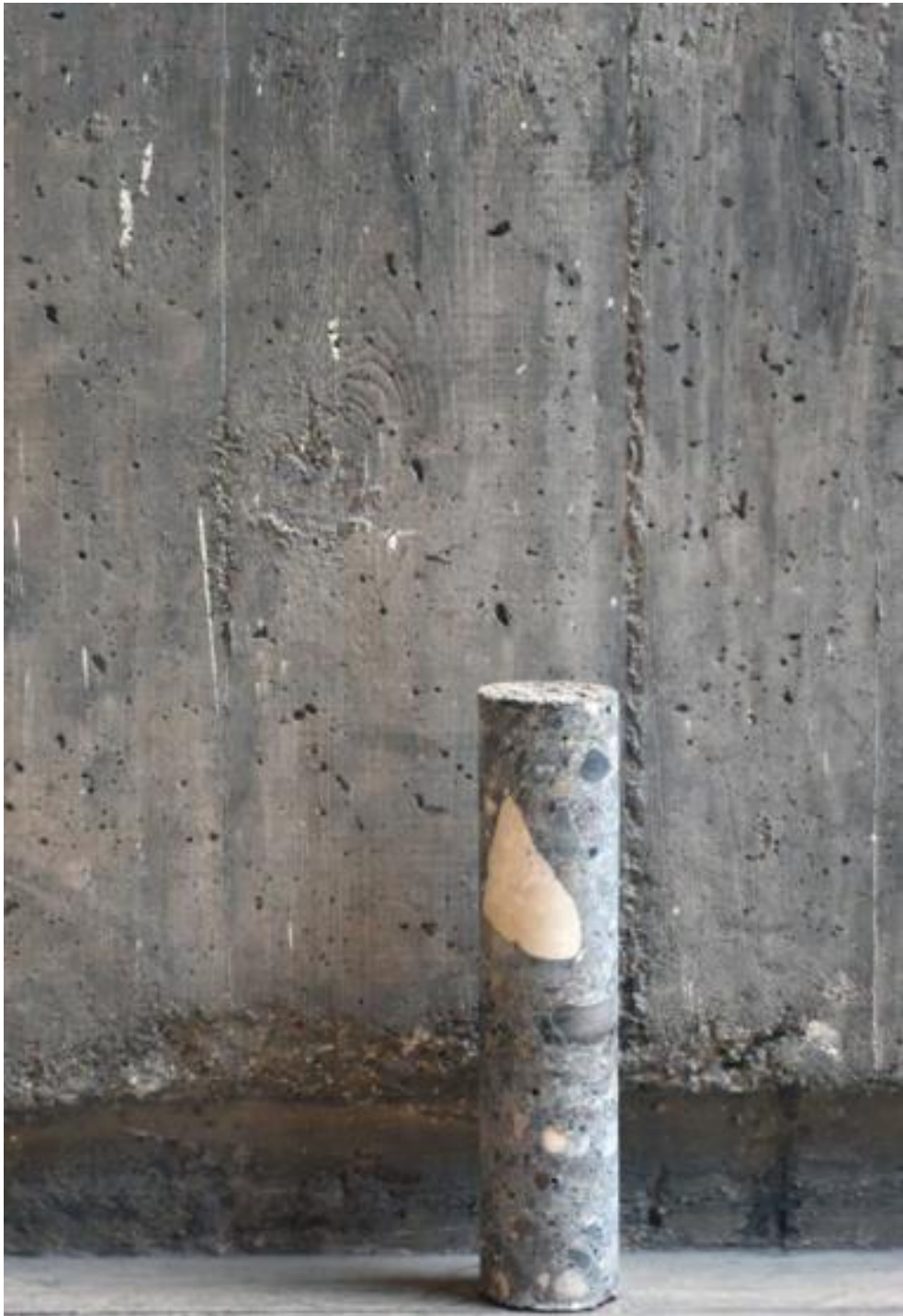
Figure 3 Core sample of the beton-brut wall section taken with the core drilling machine for conservation planning. (Also cover photograph of the Getty Report)
