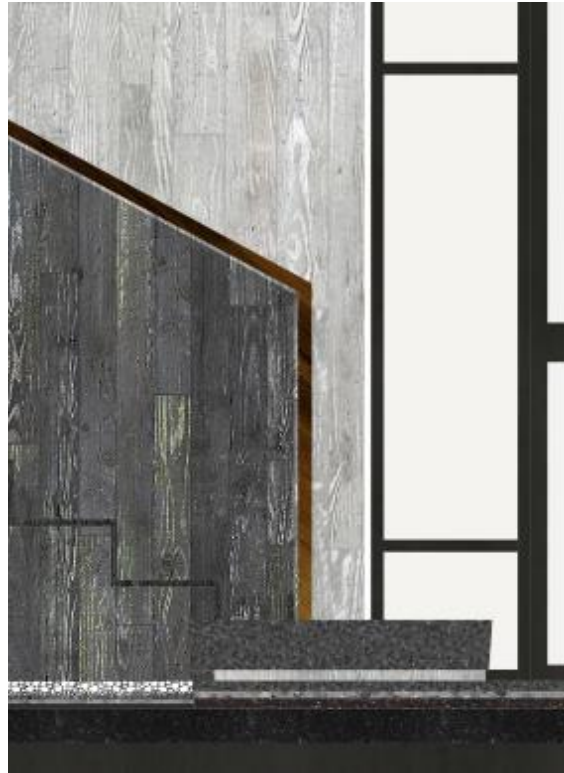
Figure 32 . Illustration detail of the staircase shows rough stone terrazzo mosaic floor, crashed stone first stair terrazzo cast, hand-made pebble stone floor decoration and joint gaps on the beton-brut balustrade covered with hornbeam handrail. (by the Author)
